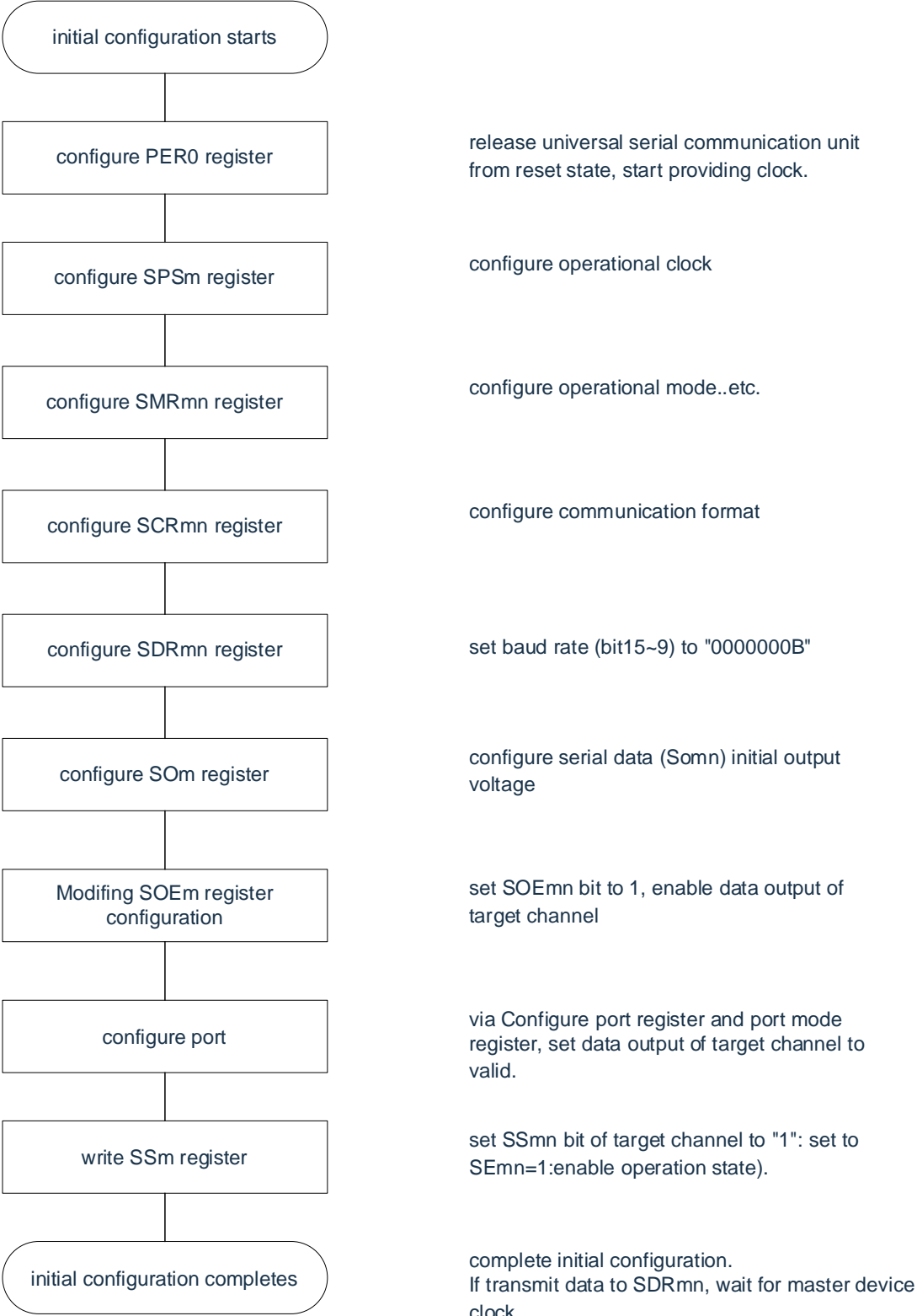
Figure 12-42: Initial setup steps for slave transmission and reception
